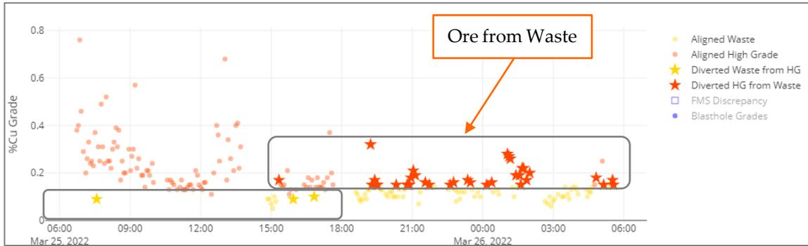
**Figure 5 Grade truck diversion client portal view at Copper Mountain mine in a day.**
