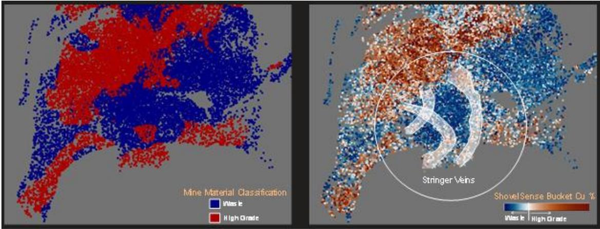
Figure 3 - The ShovelSense® bucket predicted grade view that highlights the occurrence of stringer veins not observed in the Mine Plan classification.
