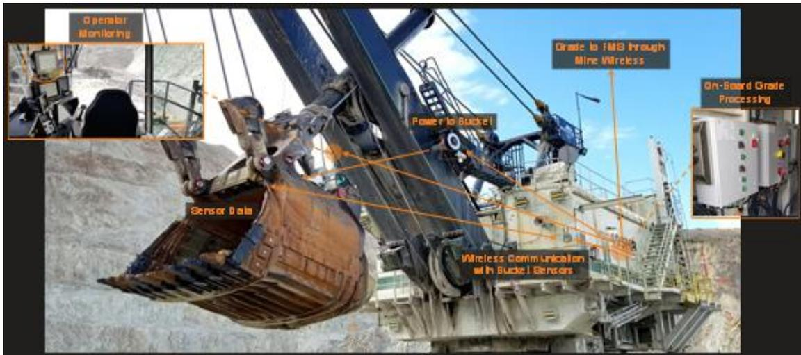
**Figure 2 - Overview of the ShovelSense® system installed on a Bucyrus 495 cable shovel**
