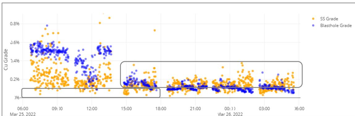
**Figure 6 Blasthole grade vs ShovelSense grade in the client portal view at Copper Mountain mine in a day.**
