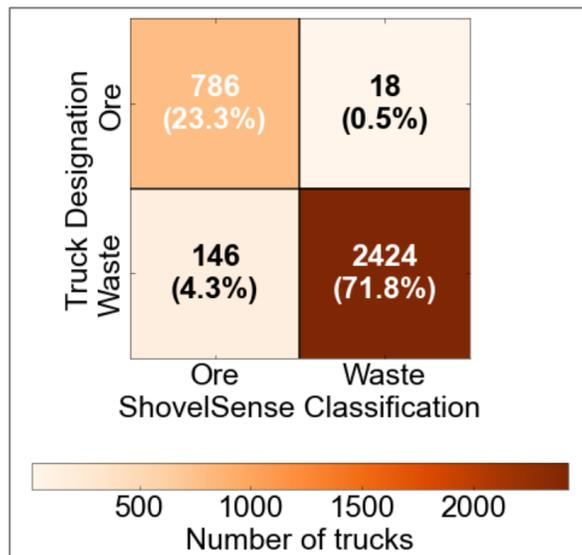
Figure 4 Truck destination classification for a specific shovel for the month of March 2022 at Copper Mountain Mine.
