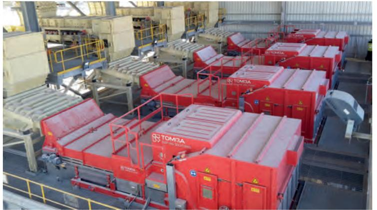
*TOMRA’s Sorting Solution division installed nine of its TOMRA COM XRT sorting units, each with an operational width of 2.4 m, to process a 1,850 t/h sorter feed at Ma’aden Phosphates’ \$560 million processing plant at the Umm Wu’ Al project in Saudi Arabia*
