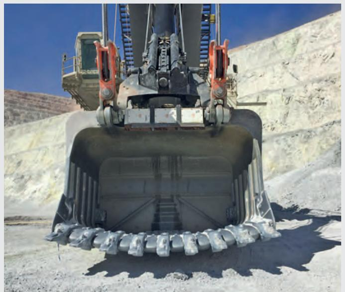
*By working at the face, ShovelSense is able to identify waste in the ore and remove it right at the pit before it incurs any extra cost, according to MineSense’s Jeff More*
